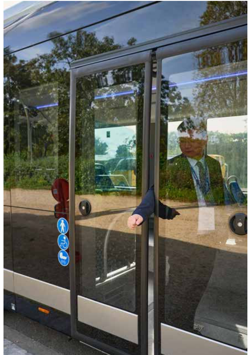
The doors of China's Yutong city bus open automatically when a person is in danger of being trapped.
